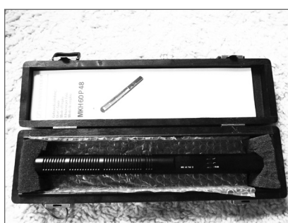
Sennheiser MKH60 Short Gun microphone phantom powered
