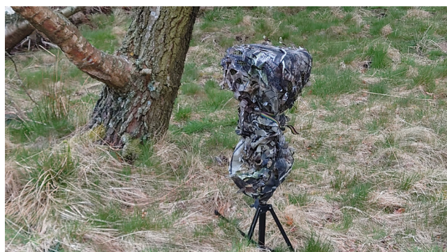
Above: Three Photos. Water resistant recorder setup. Spaced omni mics fitted in waterproof case with Zoom F3 and Battery inside. Camouflaged and Left overnight in valley
