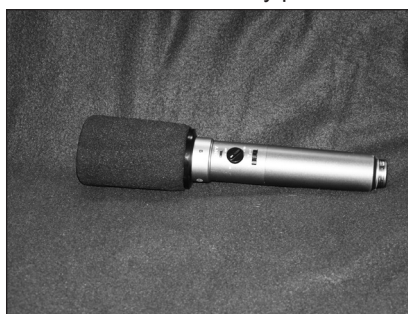
Sony ECM999 Adjustable stereo M-S Microphone Phantom or internal 'AA' battery power
