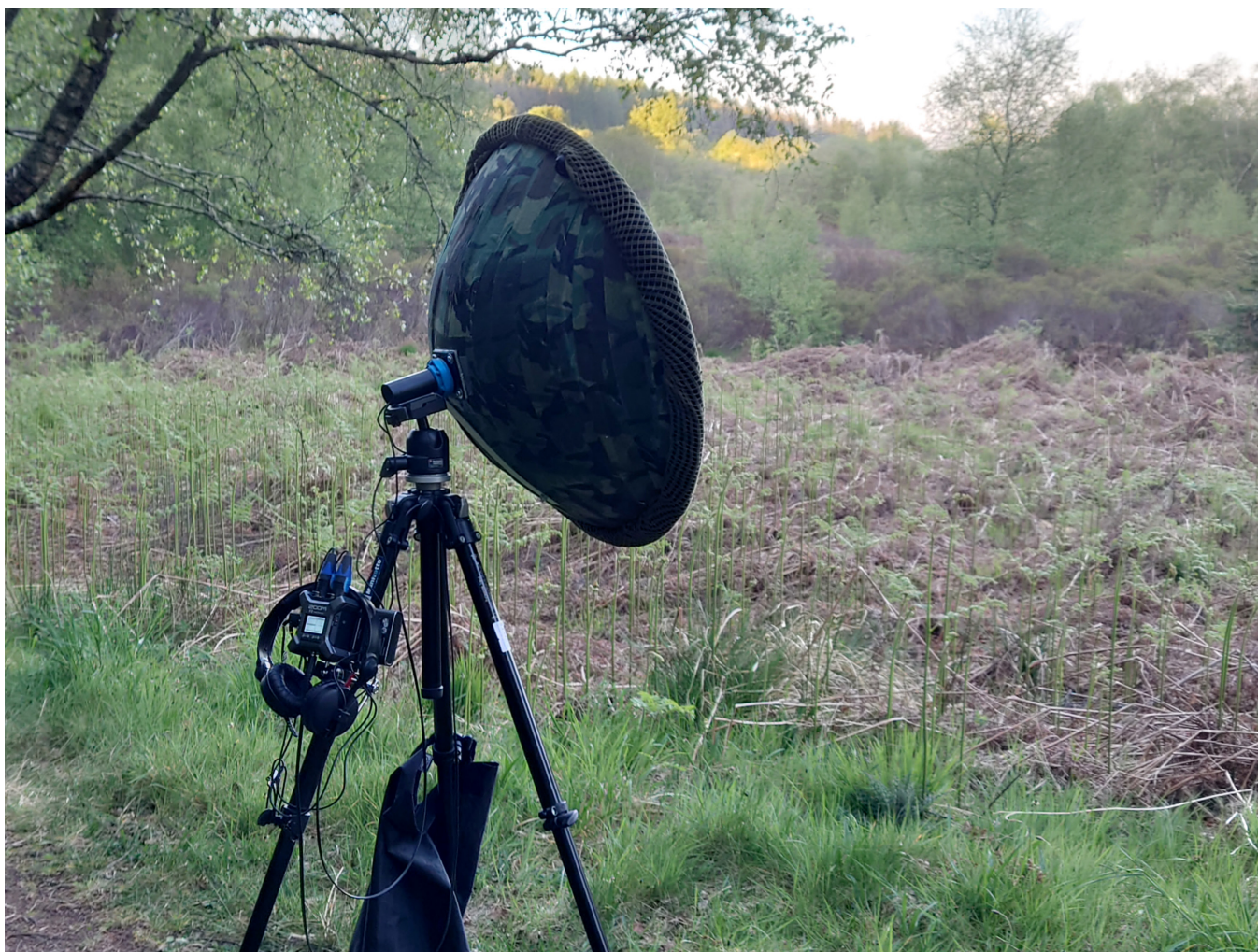
Above: Recording at Holystone Common in Northumberland on a May evening. Parabolic Reflector fitted with Zoom F3 recorder on Tripod
