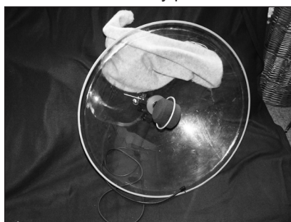
Telinga Parabolic Reflector with Stereo Microphone and wind cover. 9V 'PP' battery powered
