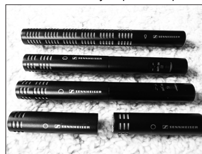
Sennheiser ME series - ME66 short gun, 2xME64 Cardioid, 2xME62 Omni + 2xK6. AA battery or phantom power
